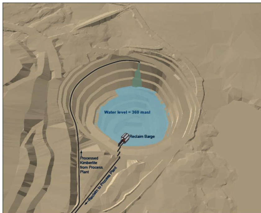
Schematic of Beartooth Pit Storage Concept Option 1: UG Mine Water and PK to Beartooth Pit (2010 to 2014) and Reclaim Water (2011 to 2014)
