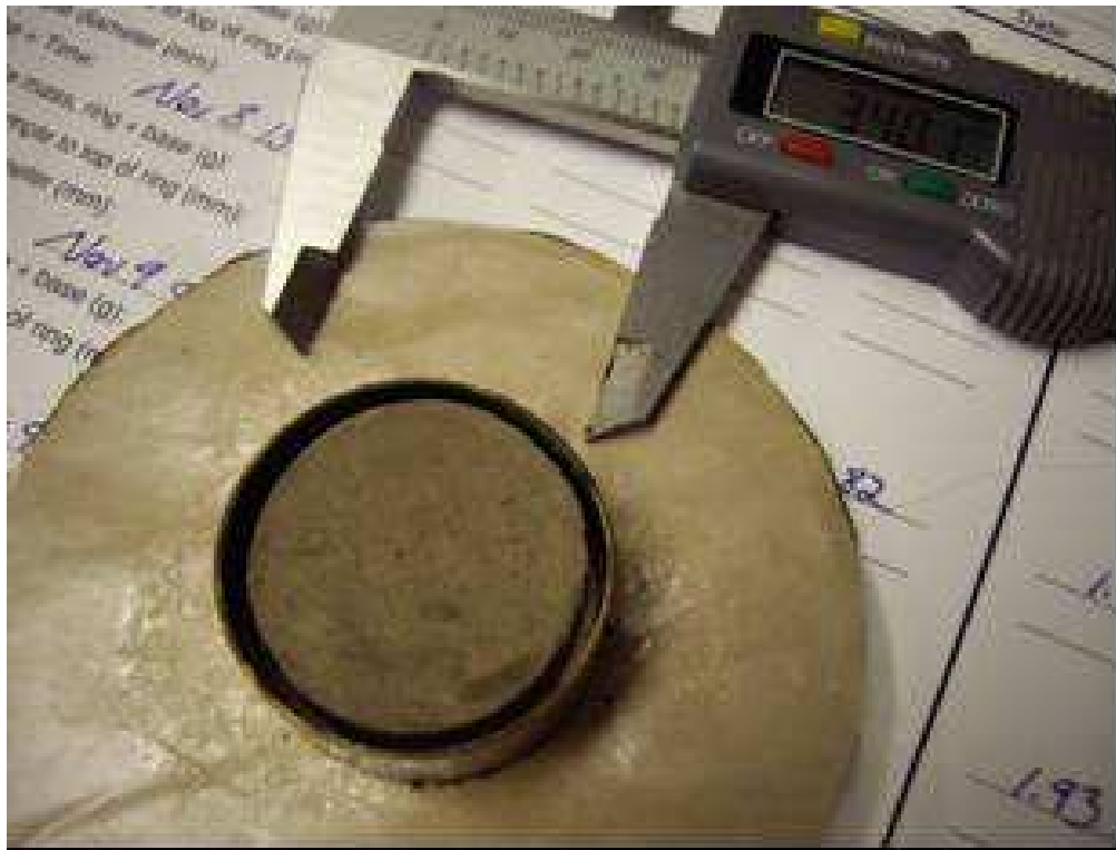
Figure 2: Digital micrometer for the measurement of the diameter and thickness of shrinkage specimens.
