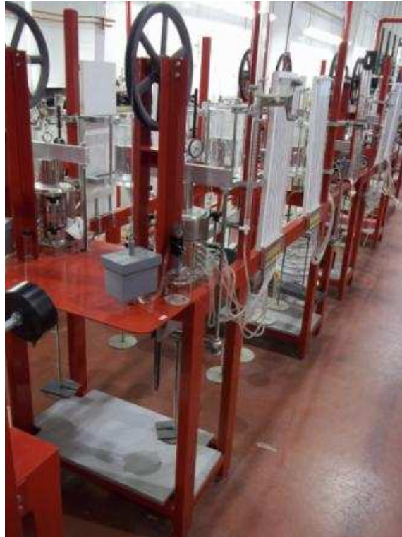
Figure 1: Slurry consolidation and hydraulic conductivity testing equipment
