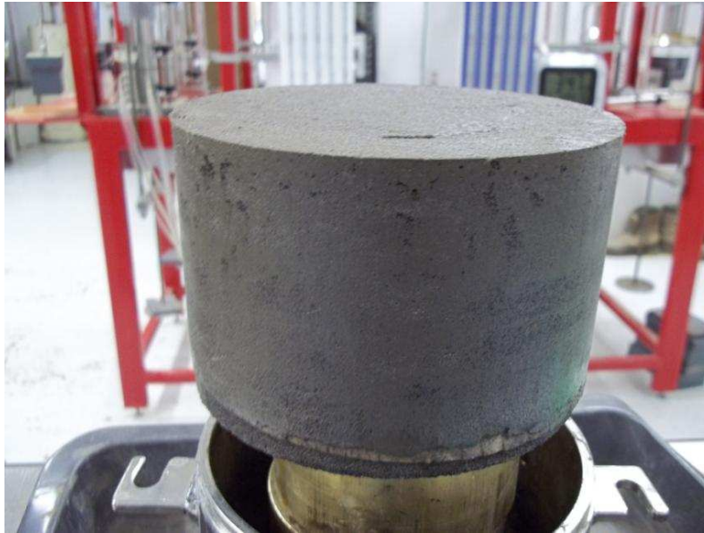
Figure 2: An extruded MFT specimen at the end of the consolidation test
