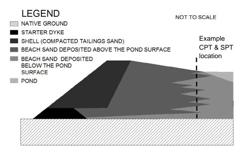
Figure 1: Schematic Illustration of an Upstream Tailings Dyke
