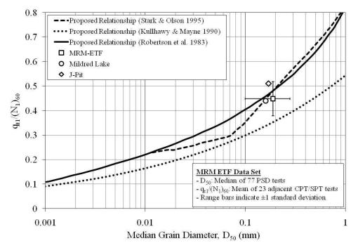
Figure 6: Comparison of q<sub>t1</sub>/(N<sub>1</sub>)<sub>60</sub> Ratios Calculated at Oilsands Mines with Standard Ratios
