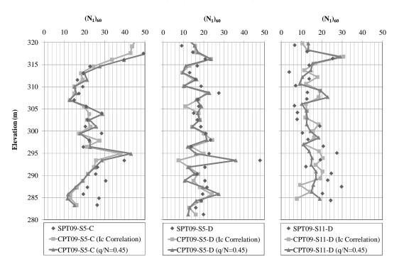
Figure 7: Comparison of  $(N_1)_{60}$  Measurements with Equivalent  $(N_1)_{60}$  Values
