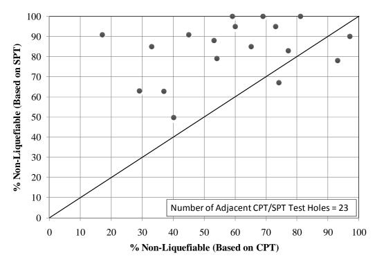
Figure 10: Effect of Non-Liquefiable Percentages Calculated using  $(N_1)_{60}$  from SPT and using  $(N_1)_{60}$  from CPT
