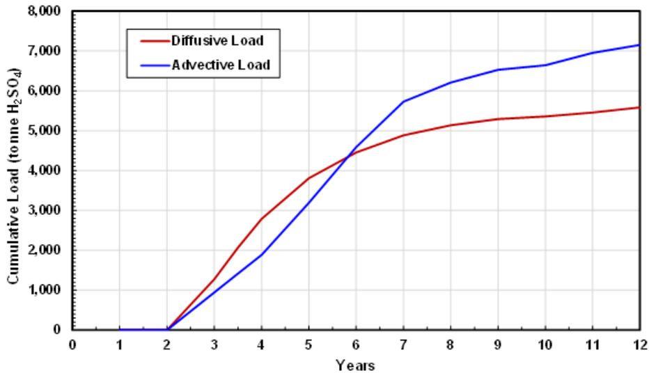
Figure 6 Cumulative loading due to diffusive and advective gas transport for Scenario 1.
