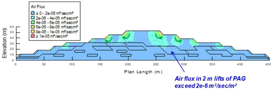
Figure 8 Air flux rate, vectors and general flow paths for Scenario 1.
