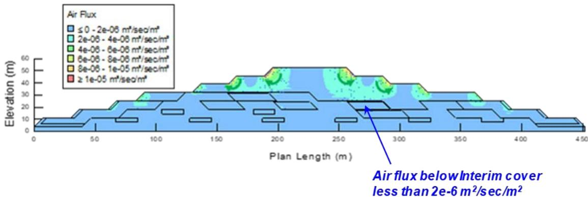
Figure 9 Air flux rate, vectors and general flow paths for Scenario 2.
