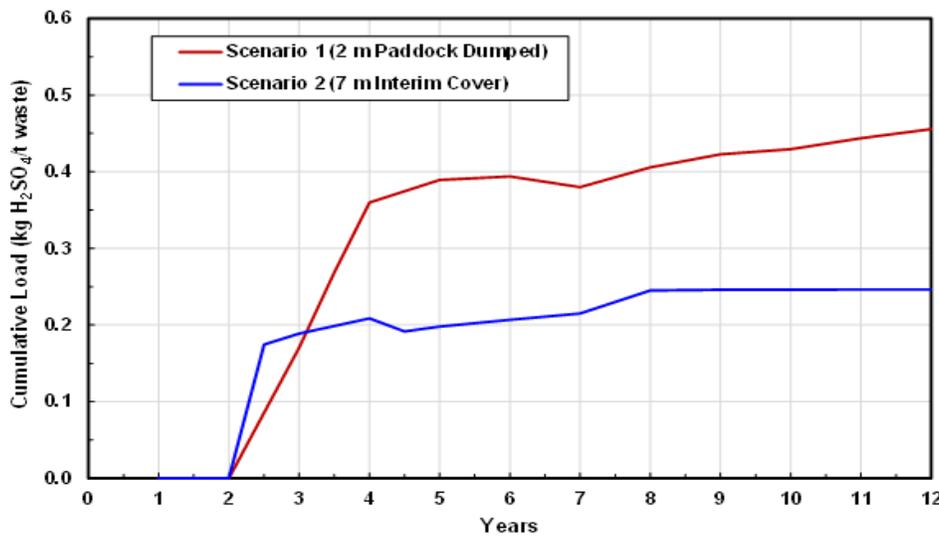
Figure 7 Comparison of cumulative acidity load per tonne of waste for Scenarios 1 and 2.
