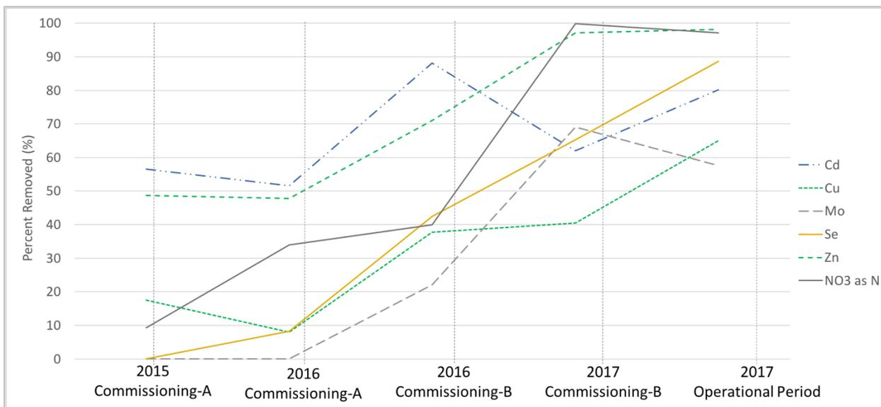
Figure 3: Average Percent Metal Removal by CWTS over Time. Percentage removals have been corrected to account for the detection limit since the percent removals were artificially low for some CoPCs (such as cadmium) because the analytical detection limit was routinely reached, thereby making it impossible to have a further extent of removal.
