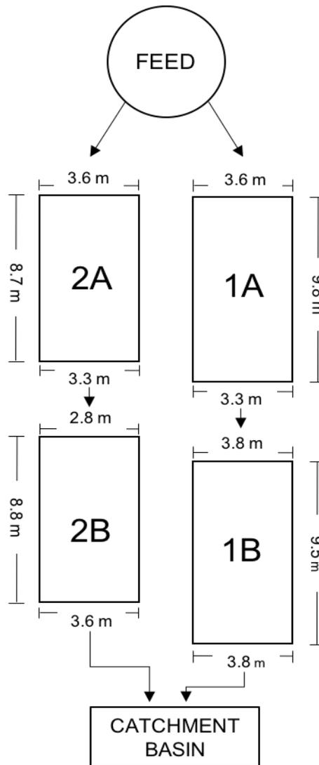
*Figure 1: Diagram of Demonstration-Scale CWTS.*
