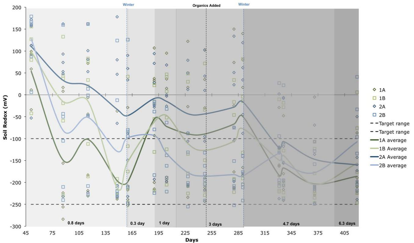
Figure 2: Soil redox potential of each CWTS cell over time (Contango, 2017). All demonstration-scale CWTS soil redox measurements are plotted. Targeted soil redox values based on pilot-scale testing are indicated with dotted lines. The blue dotted line indicates break in measurements for winter 2015 and 2016. Days and associated grey indicate the HRT (average of series 1 and 2).
