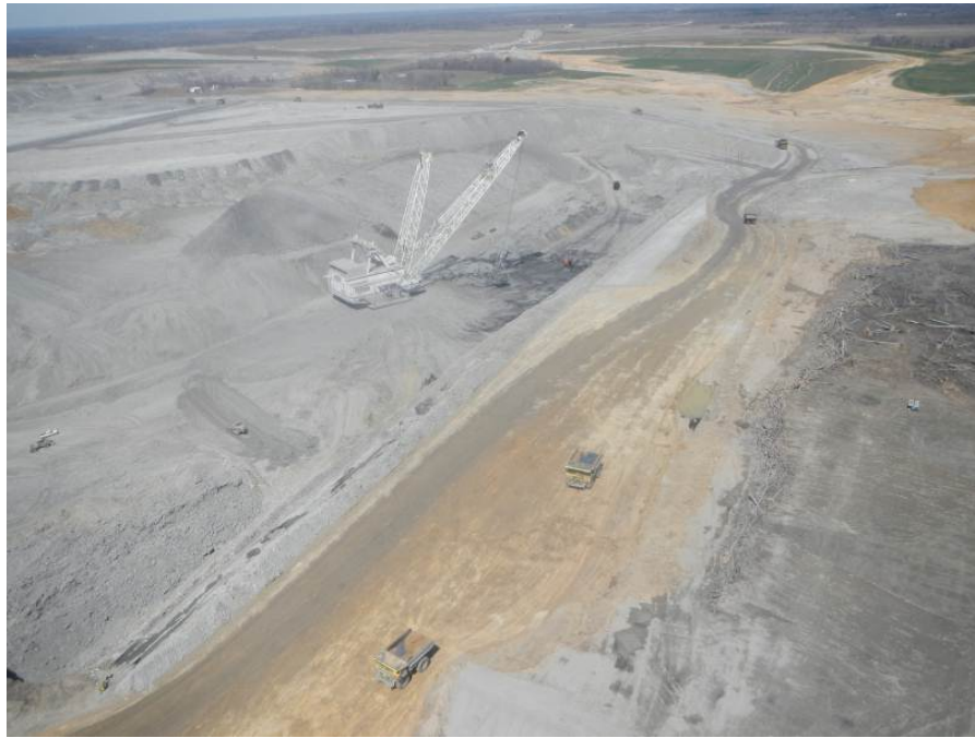
Figure 10. Dragline removing overburden from above coal seam at Bear Run Mine while end dump trucks haul topsoil for placement on top of graded cast overburden.
