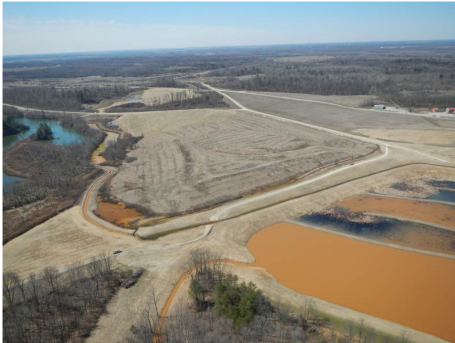
Figure 15. Gob pile covered with overburden/spoil cap near Sullivan, Indiana illustrating that acidic water can still leach for years from areas where pyritic materials are exposed to oxidation.
