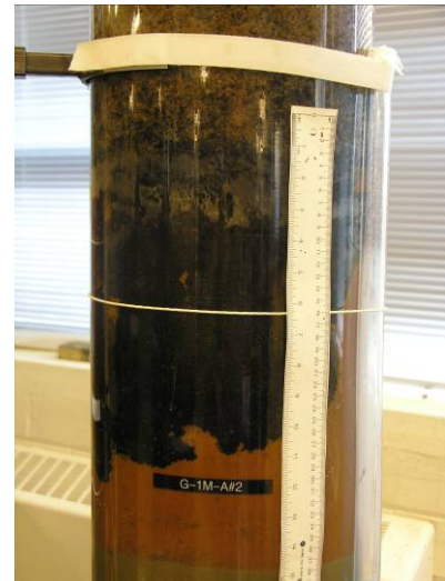
Photo 2: Close-up of black precipitate at tailings/organic interface.
