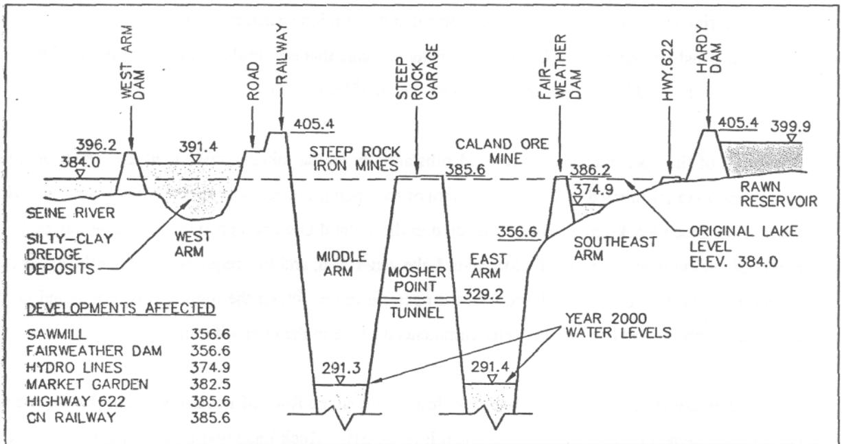
**Figure 4 - Schematic Layout of an Idealized Section through the Steep Rock Mines Area**
