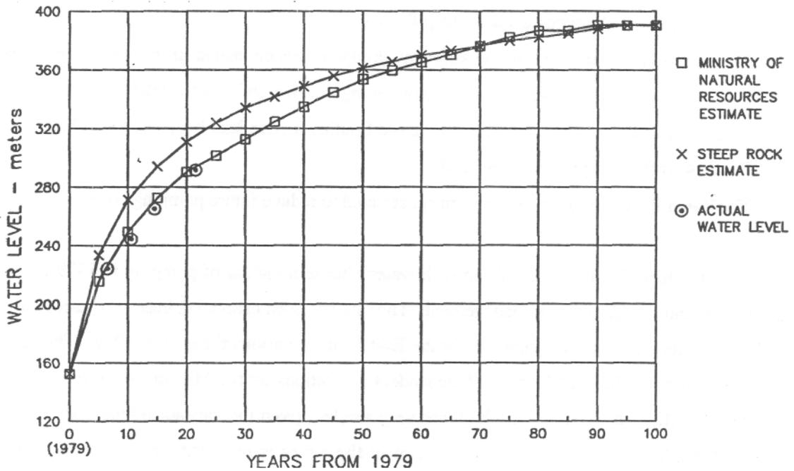
Figure 5 - Estimated rate of Water Level Rise in the abandoned mine in the East Arm of Steep Rock Lake
