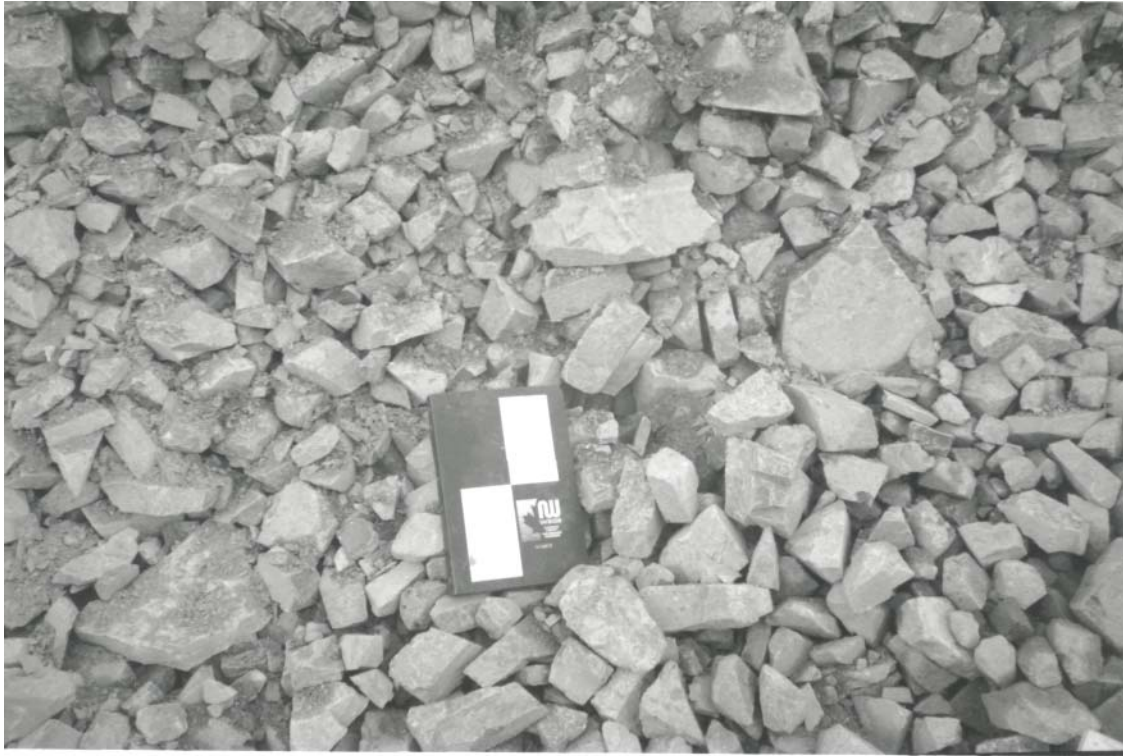
Figure No. 3 Unweathered waste rock material recently placed in the waste rock pile.
