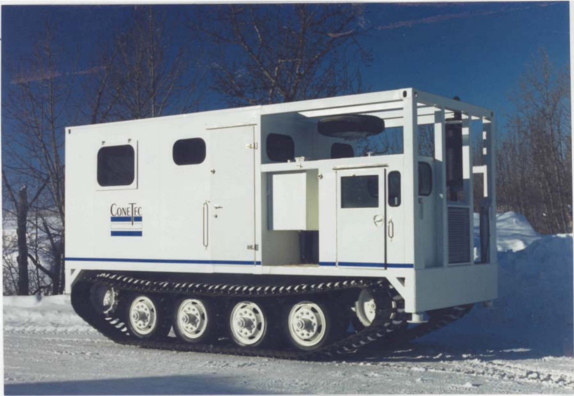
Figure 2 - Track-Mounted Cone Penetration Testing Unit
