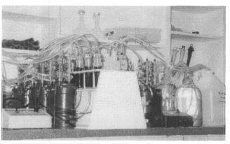
Figure 1. Column assembly used for sequential allow leaching of peat samples. Leach solution in glass bottles (on the right) was pumped through the bottom of glass columns and was collected in plastic bottles (far right).
