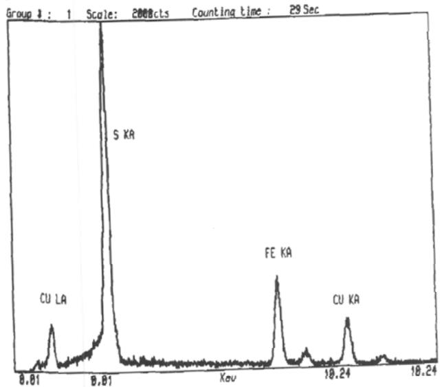
Figure 4. EDS analysis for elemental composition of a sulphide grain. Peaks for copper (CU), sulphur (S), and iron (FE) are labelled.
