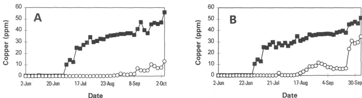
Figure 2. Copper concentration in wetland influent (•) and effluent (°). A. Small pond. B. Large pond.
