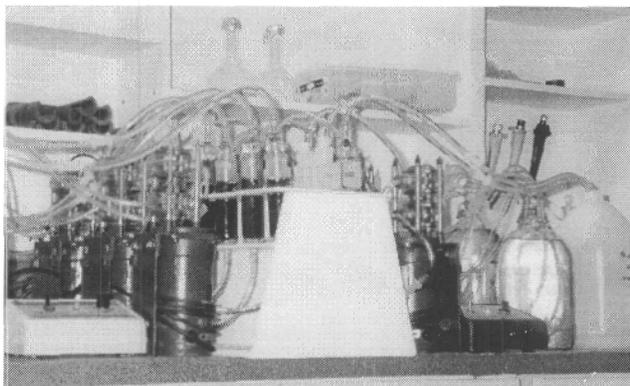
Figure 1. Column assembly used for sequential leaching of peat samples. Leach solution in glass bottles (on the right) was pumped through the bottom of glass columns and was collected in plastic bottles (far right).
