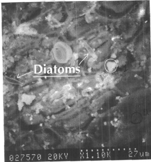
Figure 3. Photomicrograph of a sulphide grain (circled) on a carbon coated peat surface. Two algae (diatoms) are also indicated. Scale (27  $\mu\text{m}$ ) is on bottom right.
