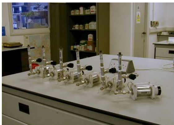
Figure 2: High pressure hydrate rocking cells for KHI evaluation experiments.
