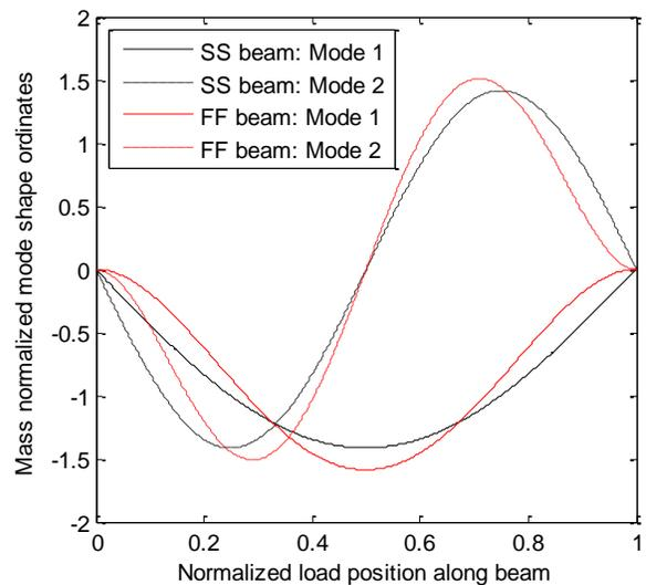
Figure 7: Mass normalized mode shapes for simply-supported (SS) and fixed-fixed (FF) beams.
