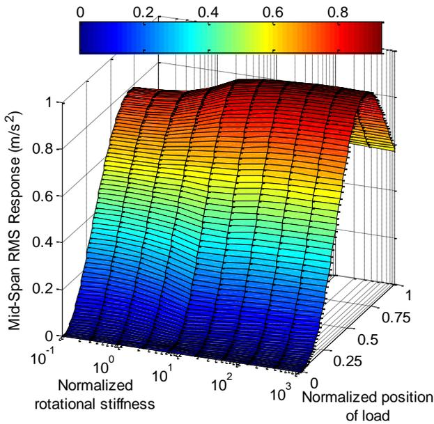
Figure 5: Complete suite of responses obtained for the RMS vibration response of the 2 Hz beams.
