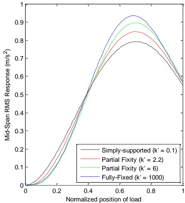
Figure 4: Vibration response of 2 Hz beams of varying rotational support fixities, subject to a constant velocity pedestrian walking force spectrum.
