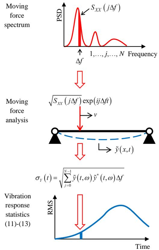
Figure 1: Illustration of the algorithm for footbridge vibration response from an arbitrary footfall force spectrum.
