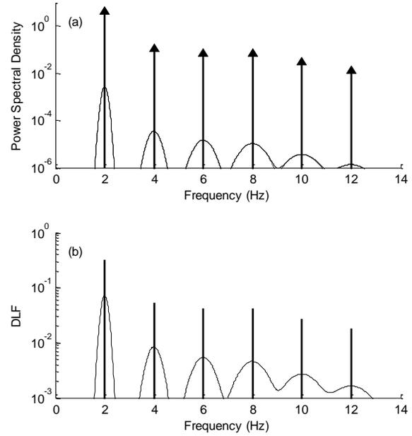
Figure 3: Simple spectral model for  $f_p = 2$  Hz showing a 5% CoV for clarity (note that 1% is used in this paper): (a) idealized walking and normally-distributed discrete spectral densities of equal energy; (b) idealized and distributed discrete DLF spectrum, transformed from (a).
