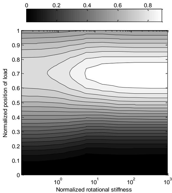
Figure 6: Alternative contour plot of the RMS vibration responses obtained for the 2 Hz beams.
