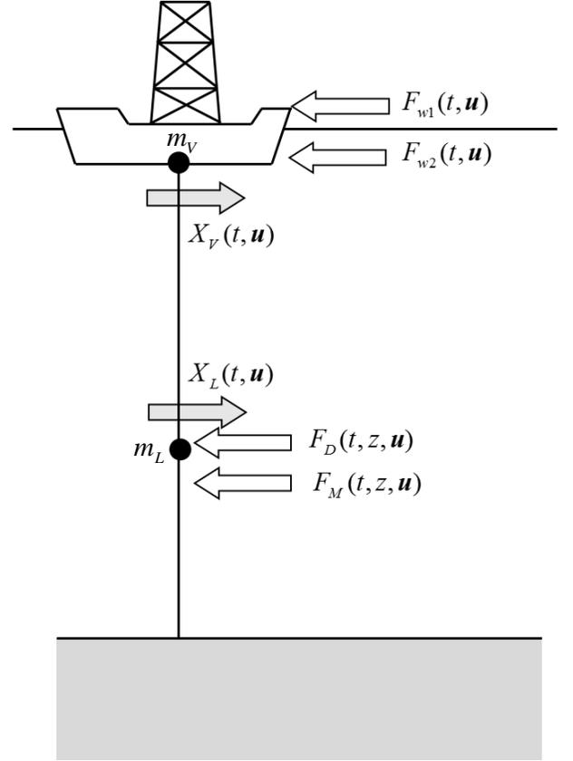
Figure 1: 2-dof simplified model of the marine riser
