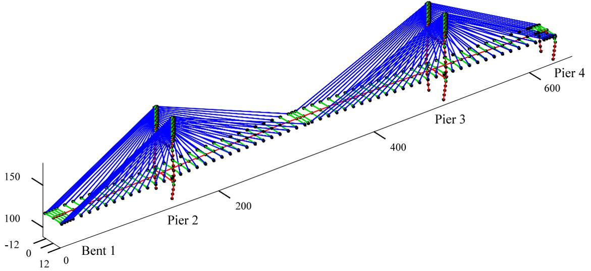
Figure 1: Finite element model of the bridge (dimensions in m); adapted from Dyke et al. (2003).
