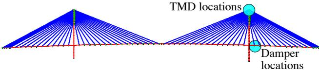
Figure 2: Finite element model (side view) of the bridge; adapted from Dyke et al. (2003).
