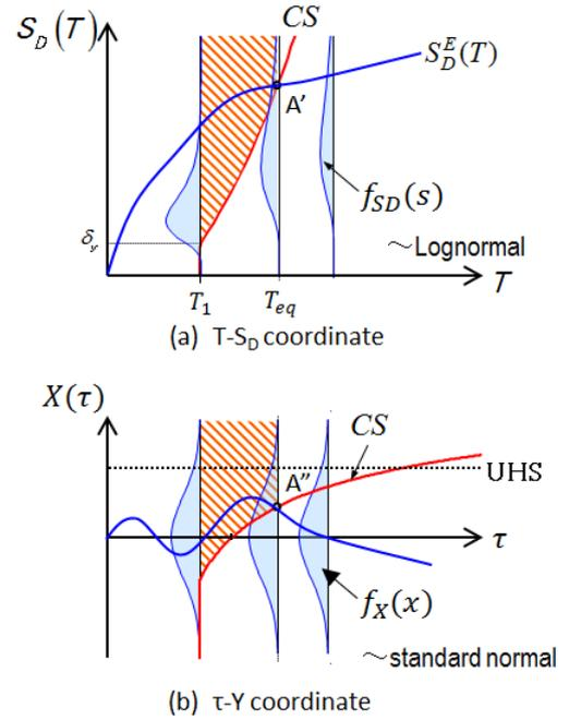
Figure 2: Schematic Illustration of CS and DS in Standard Normal Stochastic Process
