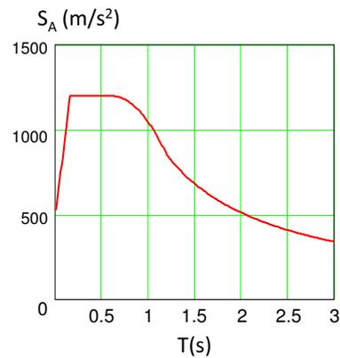
Figure 9: Design Spectrum in Japanese Seismic Provision
