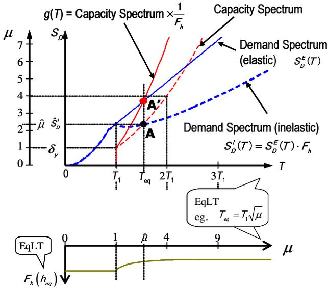
Figure 1: Capacity-Spectrum Method in  $T$ - $S_D$  Coordinate)
