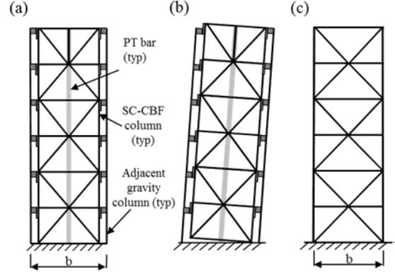
Figure 1: (a) Configuration of SC-CBF; (b) Rocking behavior of SC-CBF; (c) configuration of CBF.
