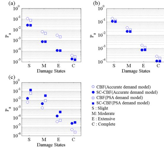
Figure 2: Annual probability of exceeding damage states for (a) structural damage ( $L_1, L_4$ - $L_7$ ), (b) non-structural drift sensitive damage ( $L_2$ ), (c) non-structural acceleration sensitive damage ( $L_2, L_3$ )
