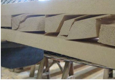
Figure 2: Rolling shear behaviour in cross layers
