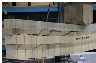
Figure 5: Failure mode in the ramp loading test
