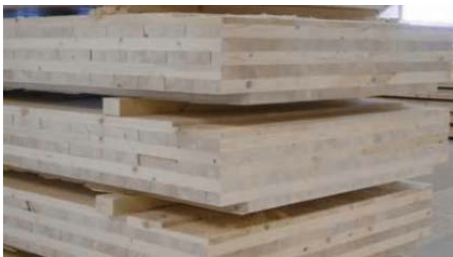
Figure 1: Layering of CLT
