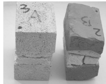
Figure 8: Appereance of deteriorated masonry samples after freeze-thaw test, Cultrone et al. (2007)
