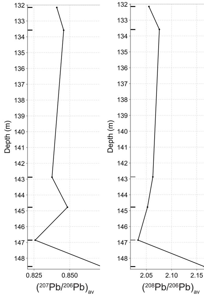
**Figure 5.9.** Stratigraphic variations in modal percentage-corrected average  $^{208}\text{Pb}/^{206}\text{Pb}$  and  $^{207}\text{Pb}/^{206}\text{Pb}$  for borehole EL-19-53. Note that the 2s error bars are not shown for clarity.
