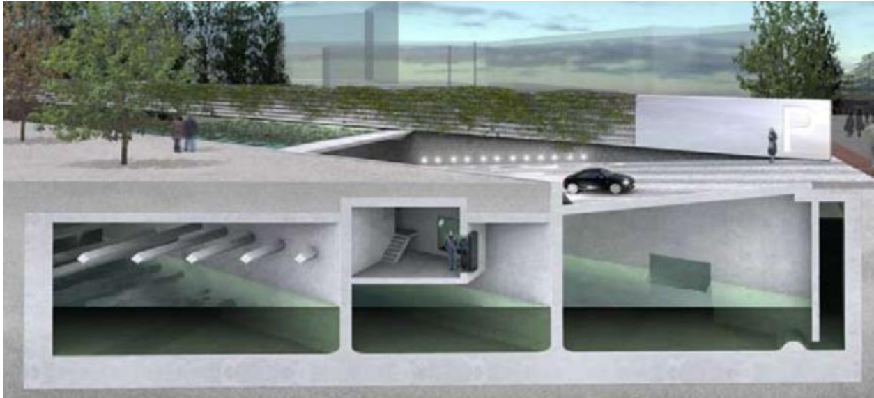
Figure 4. Multi-functional underground parking garage used as a reservoir for floodwaters and storm waters (Aerts et al., 2009).
