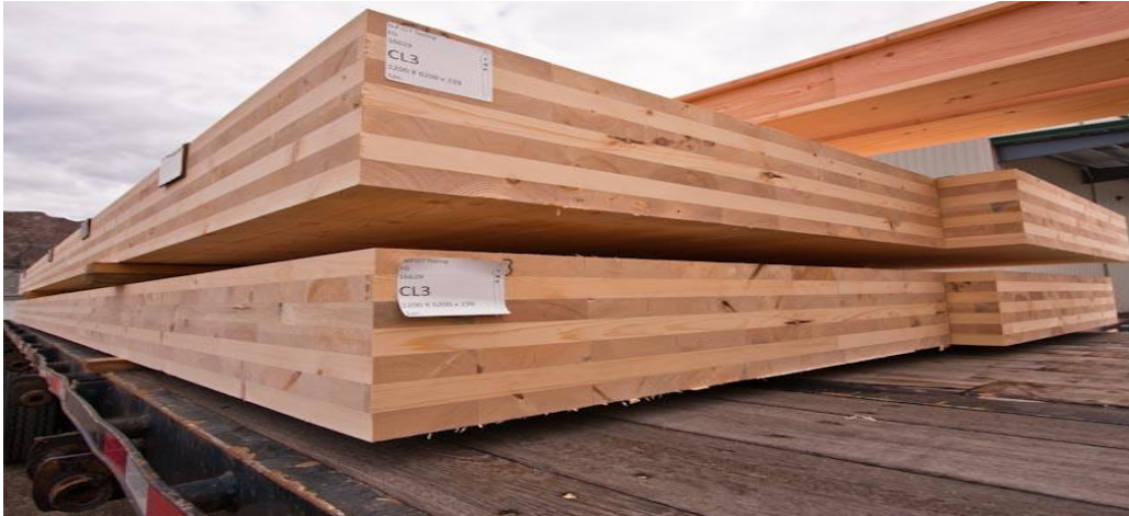
Figure 5 - 7 Layers Cross-laminated timber panels (Hunter, 2012)
