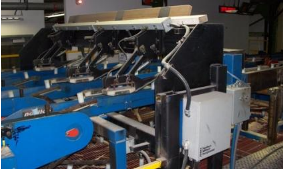
Figure 8 Dielectric sawmill moisture meter (SCS Forest Products Inc., 2012)
