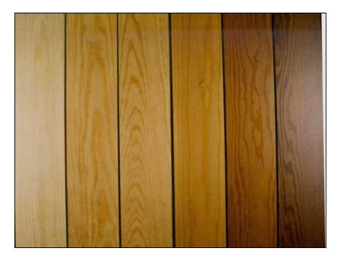
Figure 4 Hues of Heat Treated Pine from 120°C to 220°C at 20°C intervals (Thermowood)
