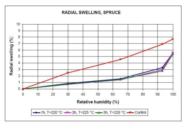
Figure 5 Radial Swelling of Thermally Treated Spruce (Thermowood)
