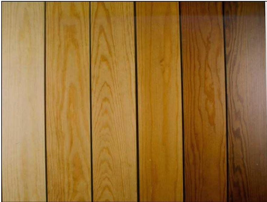
Figure 4 Hues of Heat Treated Pine from 120°C to 220°C at 20°C intervals (Thermowood)
