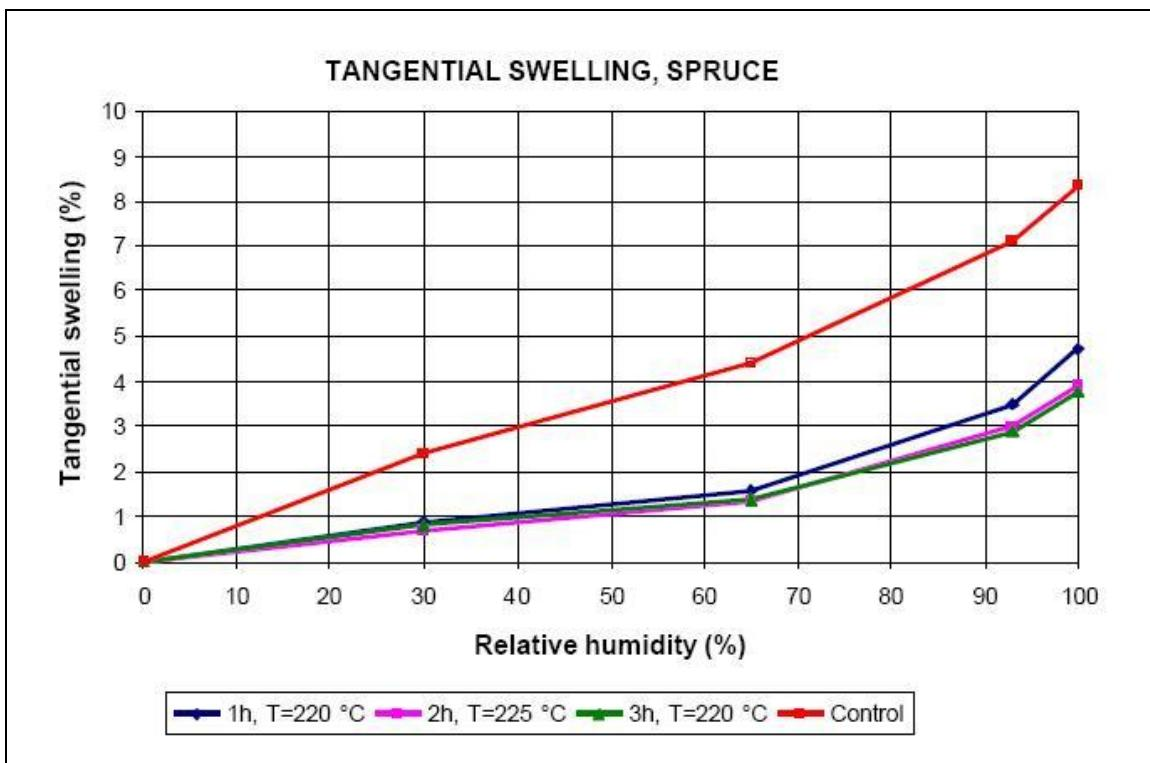
Figure 6 Tangential Swelling of Thermally Treated Spruce (Thermowood)
