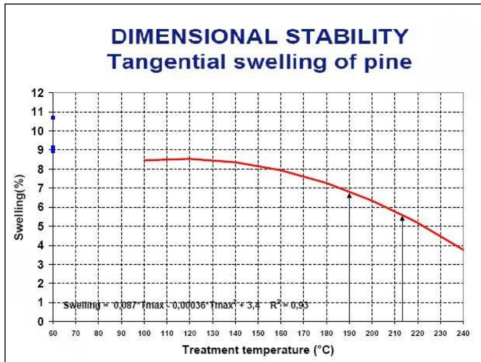
Figure 7 Tangential Swelling to Treatment Temperature (VTT)
