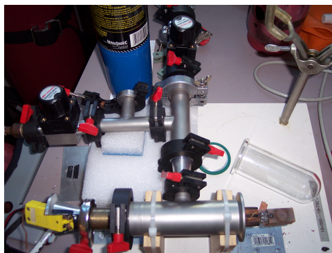
Figure 2.14: The lightbulb annealer used in this project. The chip is placed on the copper sheet in the bottom right, which surrounds a projector-bulb. The voltage to the bulb can be adjusted, which adjusts the amount of heat it releases and therefore the temperature of the chip, which is constantly measured. The chip and heat source can be encased in a glass tube and put into vacuum or into forming gas.
