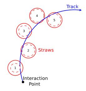
**Figure 2.2:** A charged particle path passing through five straws to create a track. The solid red circles are straw walls, dashed red circles are drift circles, and the blue path is the reconstructed track of the particle, which follows the drift circles. The interaction point is where the actual event occurred, and the straws are numbered to show the order in which the charged particle passed through them.
