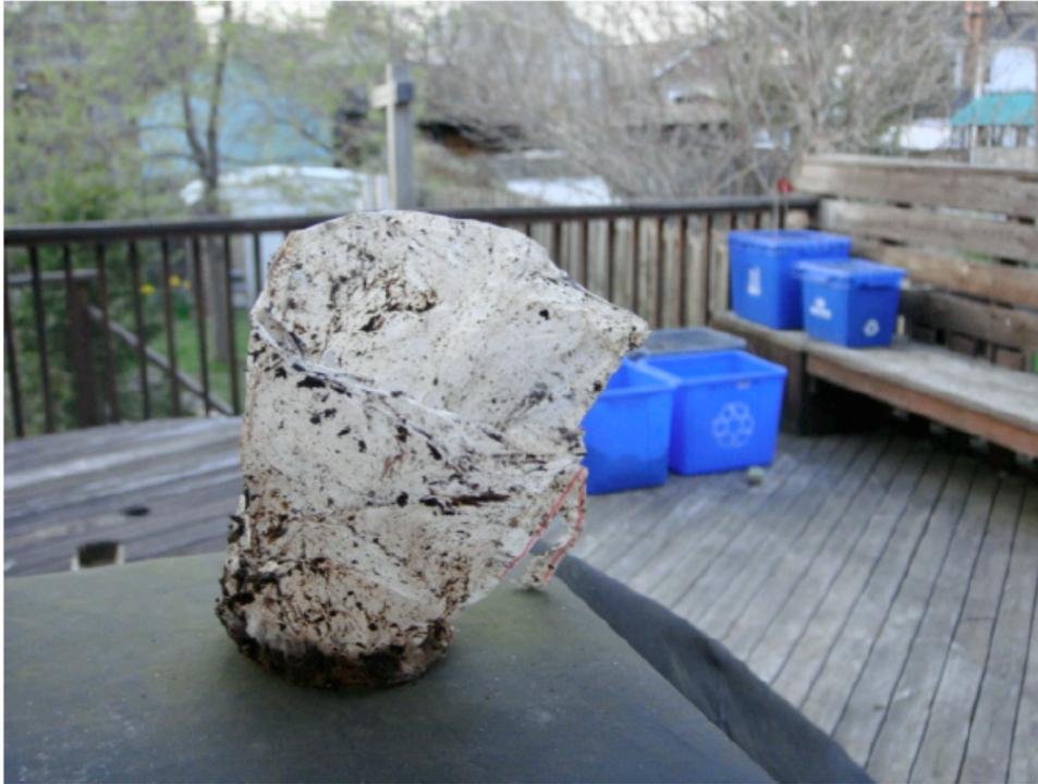
*Figure 1.* Polyethylene lining that remains after the paper of paperboard cups biodegrades (Ziada 2009).
