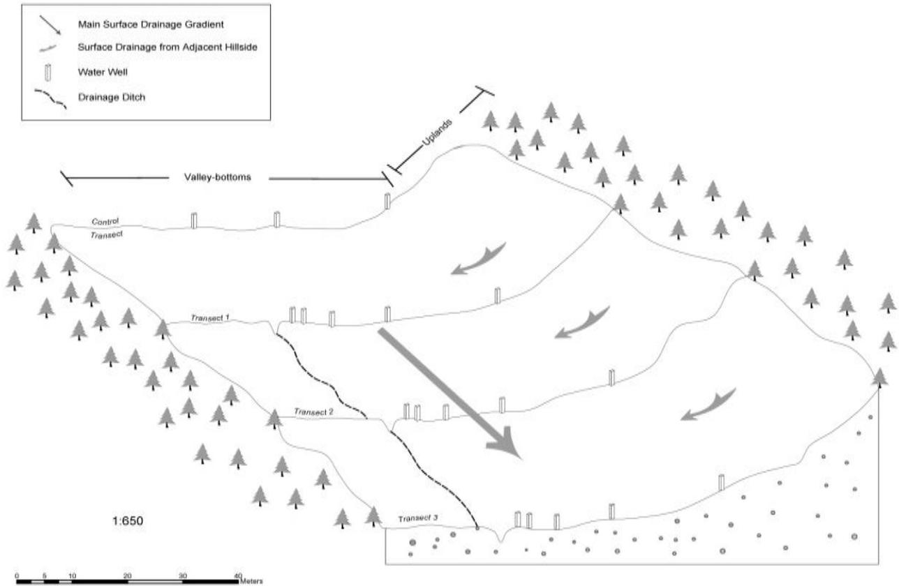
**Figure 1.** Site layout showing location of waterlogged soils and ditchline. Transects were established to install wells in various distances from the ditchline.
