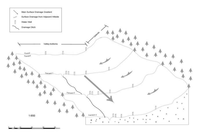
**Figure 1.** Site layout showing location of waterlogged soils and ditchline. Transects were established to install wells in various distances from the ditchline.
