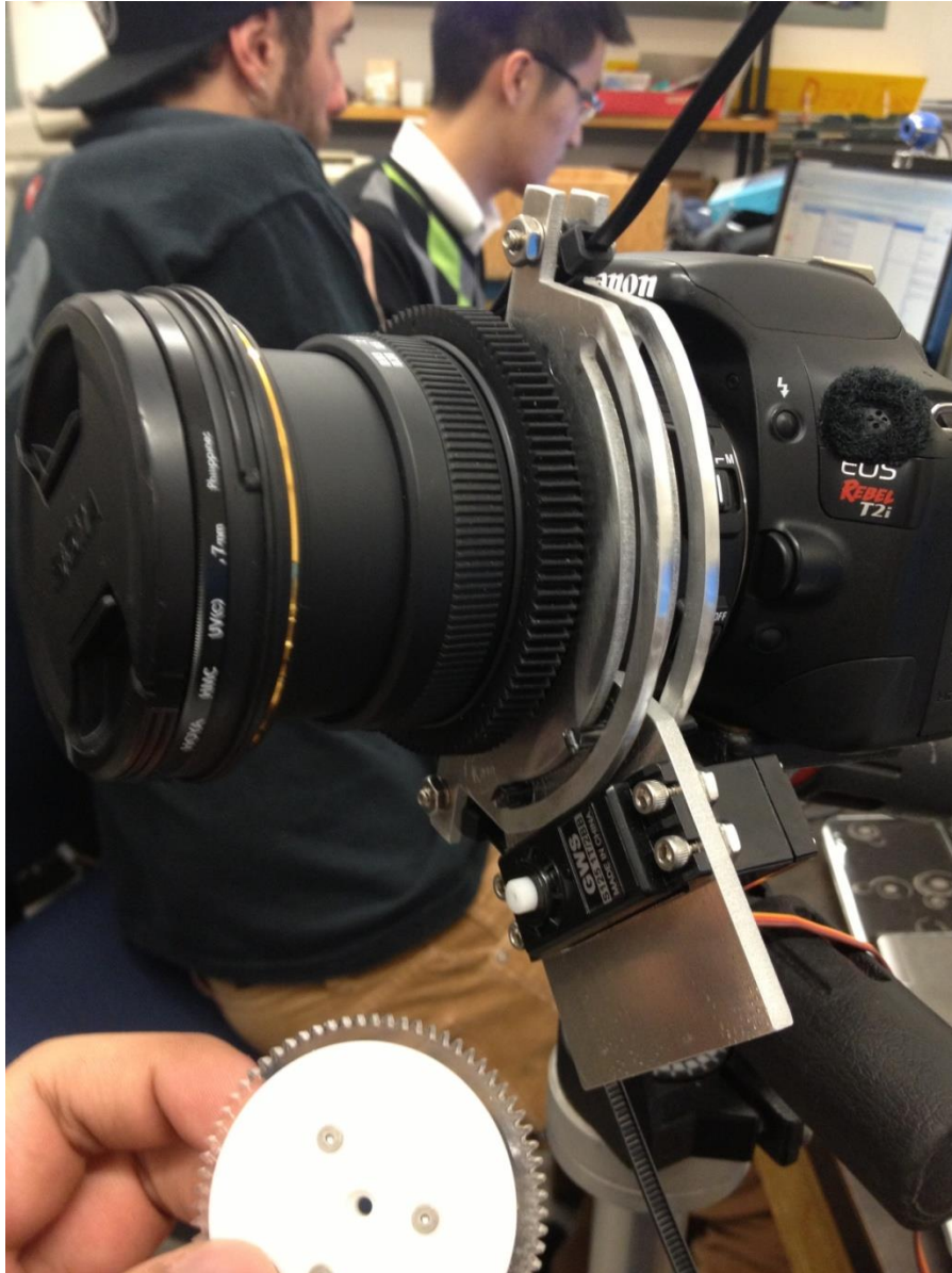
Figure 8: Size of gear to large
