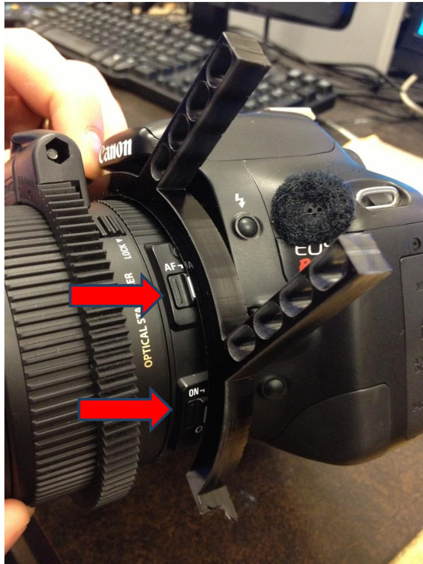
Figure 6: Blocking of Button Functionality (first prototype)
