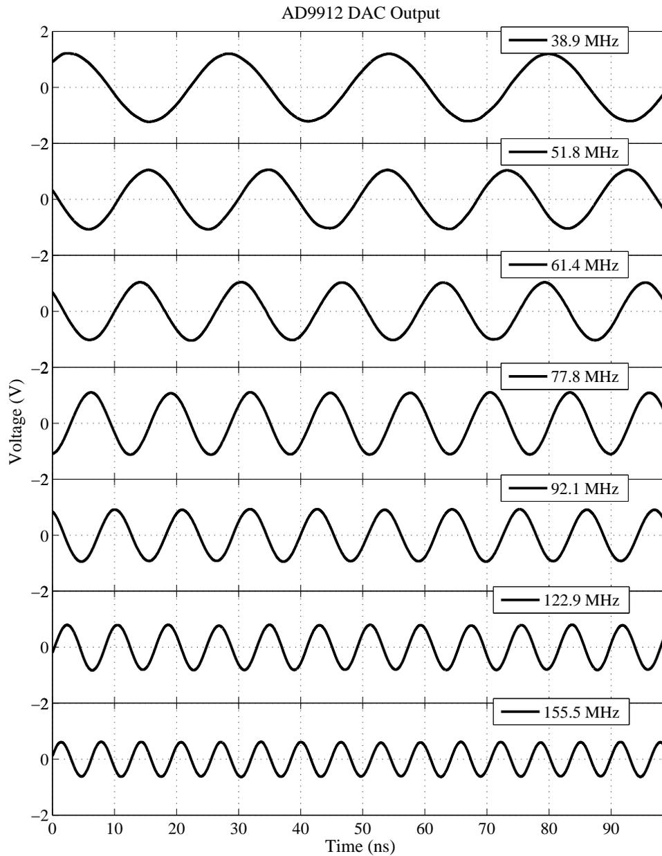
Figure 2.7: Filtered DAC output. Measured with a 60MHz, 1GS/s oscilloscope. The frequency levels were set with the AD9912 startup pins and are preset to one of 7 frequencies as defined in the AD9912 datasheet.
