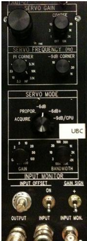
Fig 26: This figure shows a clearer picture of the front panel of the JILA PI controller. Here the knobs are used to change the values of the various parameters. What these parameters mean are discussed in detail in the “Theory” section.
