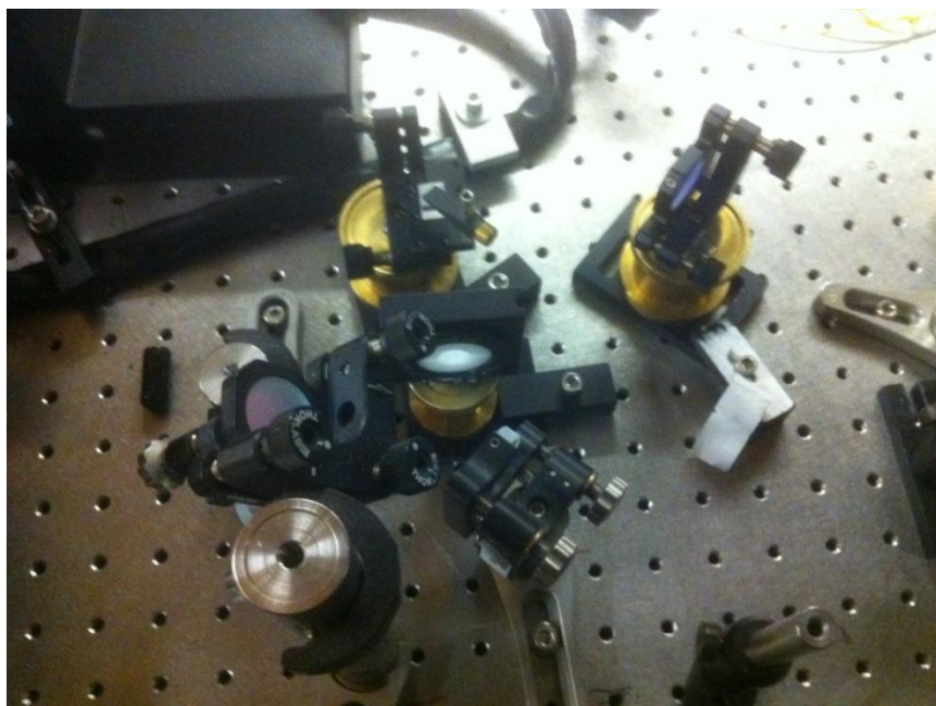
Fig 16: The beamsplitter setup that splits the light from the functioning Ti:Sapph.
