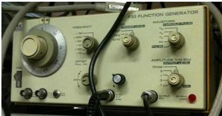
Fig 22: This figure shows a standard function generator. This function generator is used to control the piezoelectric element inside the cavity, thereby changing the length of the cavity. This function generator can also generate a sawtooth wave, which is used to sweep the cavity across different lengths in order to locate the length at which a resonant peak exists in the cavity.
