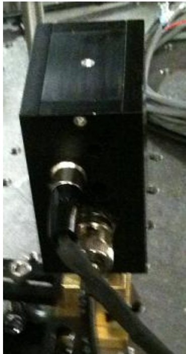
Fig 30: This figure shows the photodiode, a device that converts the intensity of the laser beam into a voltage value.
