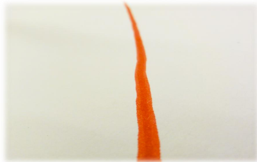
FIGURE 28: DRAWING WITH 3MM WIDE MARKER PEN
