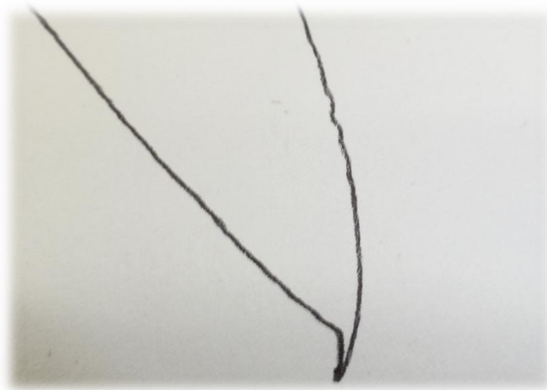
FIGURE 29: DRAWING ANOMALY CAUSED BY IMPERFECT GEARING
