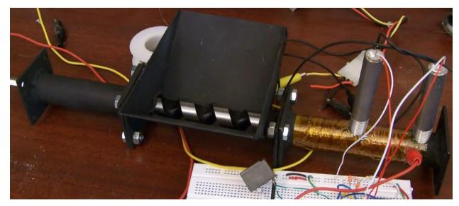
Figure 2 - Homemade plastic extrusion system (Screen capture of Youtube video by web4deb, see reference "Homemade Plastic Extrusion System", 2010)
