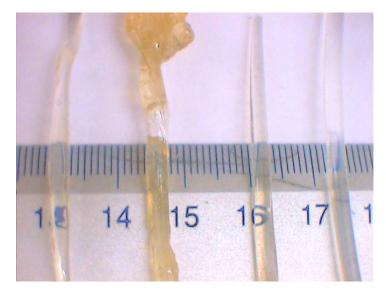
Figure 6- Extruded PLA filaments, far right shows commercial filament for comparison.
