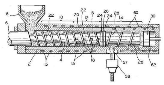
Figure 1- Schematic of plastic extrusion device. Hopper at top left feeds plastic granules into the screw which conveys them through the heating zone and forces the molten plastic through the die. (Adapted from US Patent 4118163, Plastic Extrusion and Apparatus, by Soo-II Lee)
