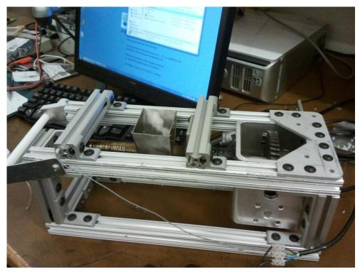
Figure 3- Plastic extruder prototype. Gearbox at right, hopper in center, and outfeed roller at far left.
