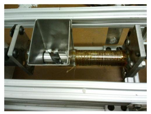
Figure 4- Close-up of hopper and heating tube with NiChrome heating wire.
