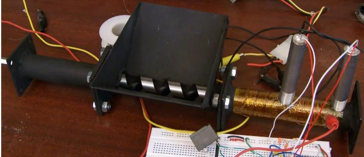
**Figure 2 - Homemade plastic extrusion system (Screen capture of Youtube video by web4deb, see reference “Homemade Plastic Extrusion System”, 2010)**
