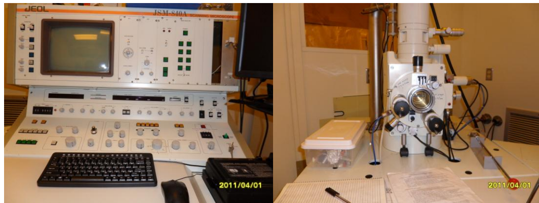
Figure 16. Scanning Electron Microscope at AMPEL (equipped with electron beam lithography functionality). Left: Control Panel; Right: Microscope
