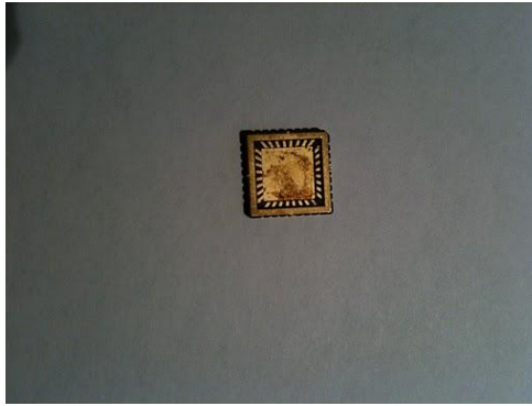
Figure 5. Integrated Circuit Socket Compatible with the Wire-bonding Machine at AMPEL
