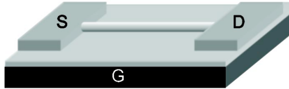
Figure 4. A Diagram of Single-nanowire Transistor (S is source; D is drain; and G is gate) [13].
