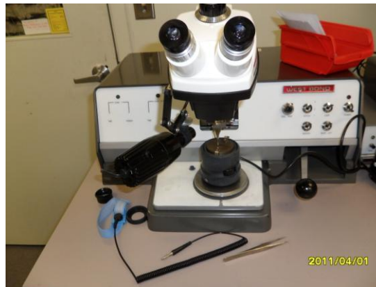
Figure 19. Optical Microscope at AMPEL (max magnification 1000x)
