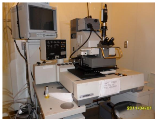
Figure 13. Karl Suss Aligner (used for UV exposure)
