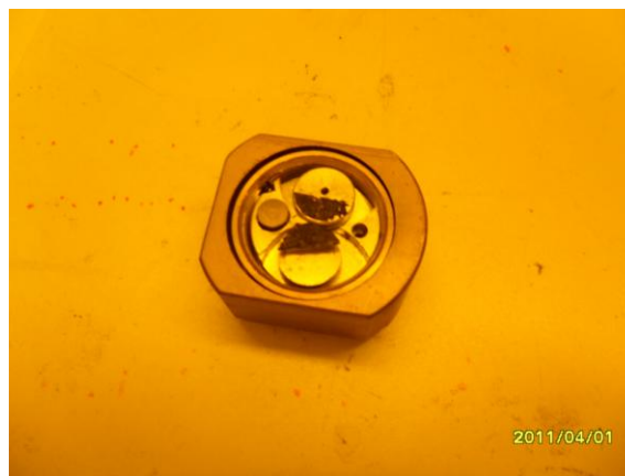
Figure 17. Sample Holder for Scanning Electron Microscope at AMPEL
