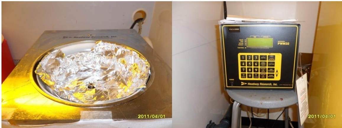
Figure 12. Headway PWM32 (Spinner) Used to Apply a Uniform Layer of Photoresist (right: the sample is held in place in the middle by a vacuum pump; left: the programmable controller for Spinner).
