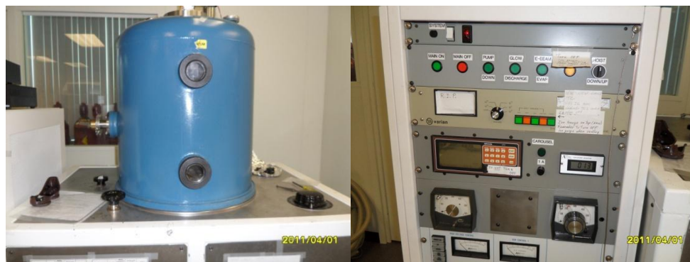
Figure 14. Evaporator at AMPEL (right: vacuum chamber; left: control panel)
