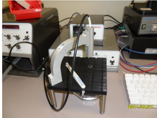
Figure 18. Filmmetrix F20 (measures PMMA thickness)
