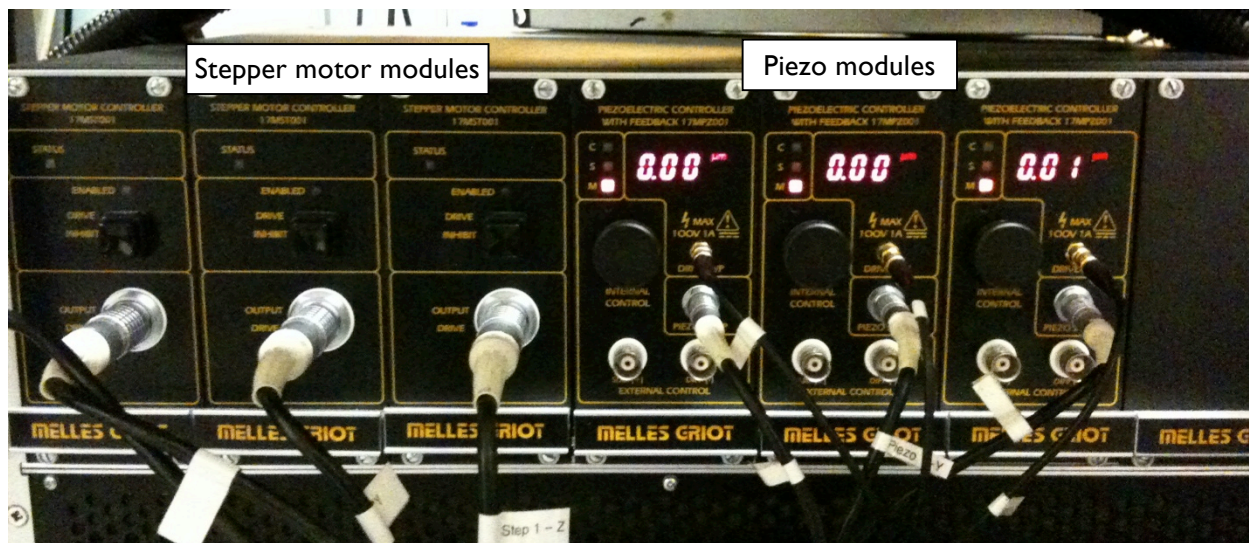
Figure 5: Stepper motor and piezo control module
