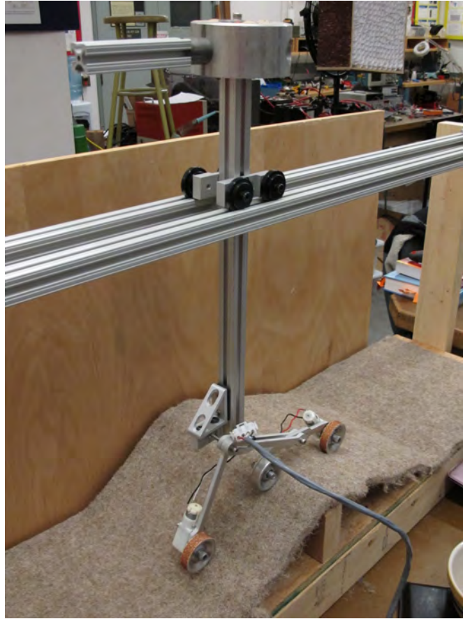
Figure 2.2: Overhead Linear Track and Vertical Support System
