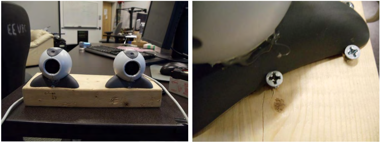
Figure 4 (a) Two Logitech QuickCam Messengers are positioned side by side for triangulation. (b) The cameras are pinned to the wooden block using additional screws.
