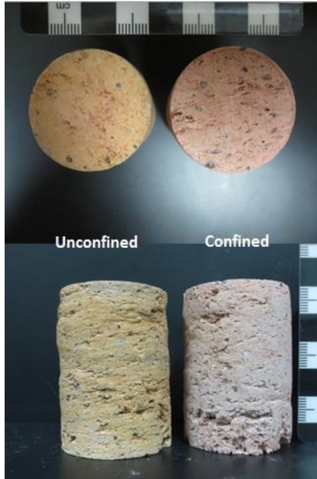
Figure 8. Two cores deformed to 30% strain. The unconfined core shows minor localized strain but no major bulging. The confined core is oxidized red due to the alumina.
