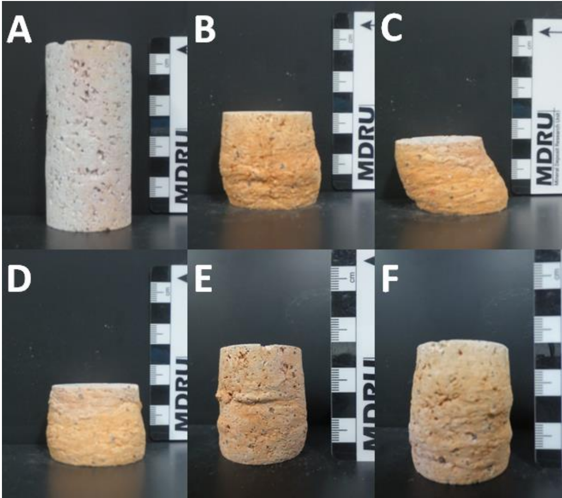
Figure 15. A) 8 cm core before deformation. B) Core deformed to 50% strain in constant displacement. C) and D) Core after 3559 N constant load experiment. E) and F) Core after 1334 N constant load experiment.
