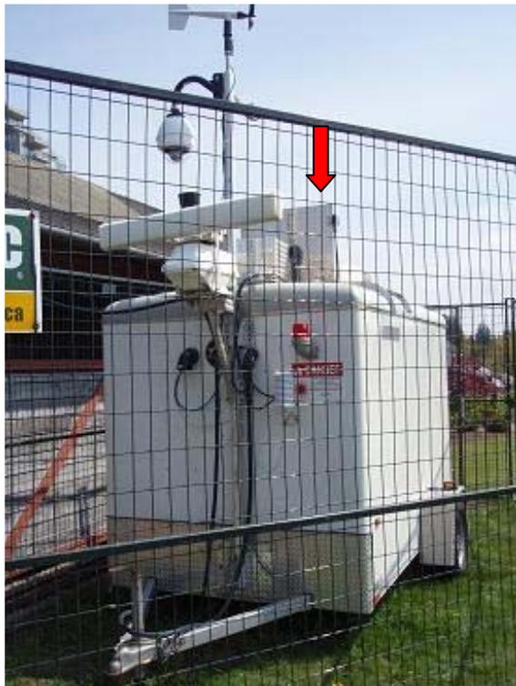
**Figure 4.** CORALNet-UBC lidar in a modified cargo trailer, located on UBC campus, Vancouver. The red arrow points to the roof hatch that closes at the onset of precipitation, causing the lidar to effectively shut off. Modified from CORALNet (2010).
