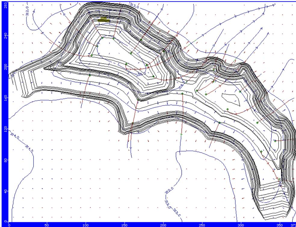
Figure 13: Flow velocity vectors and pathlines for defined water table 1.5m deep,  $K_{xy} = 5 \times 10^{-4}$  cm/s. Reduction of the  $K_{xy}$  to  $1 \times 10^{-5}$  cm/s yielded similar flow vectors but at a reduced maximum velocity of  $2.3 \times 10^{-5}$  cm/s. Particles exited the hummock on the order of 14 years. Table 5 below summarizes the volume inputs for the lowered k value.
