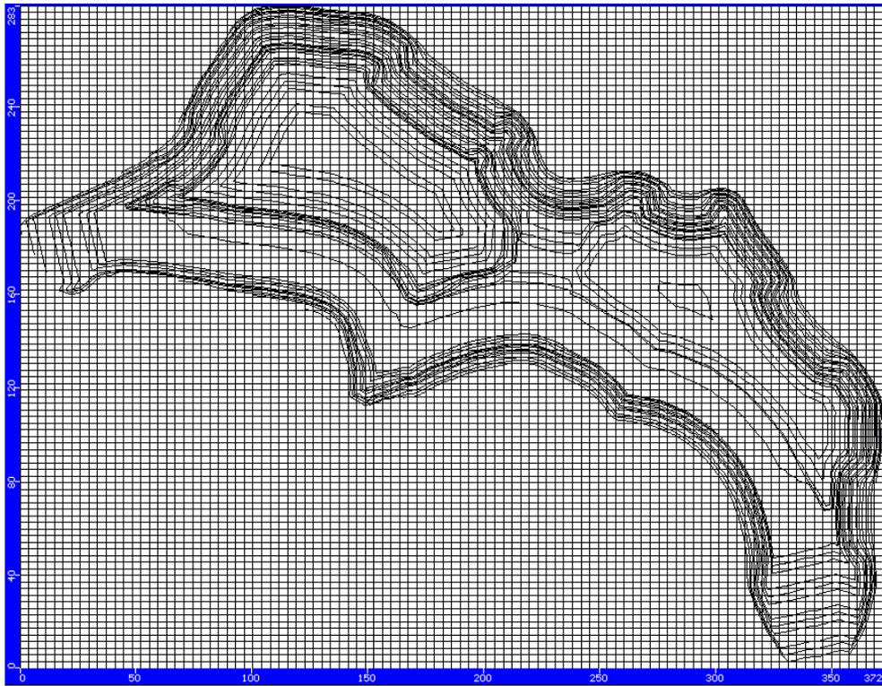
Figure 3: Numerical model grid, plan view.
