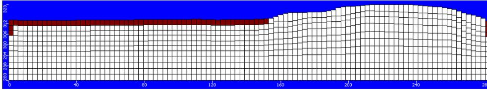
Figure 11: Constant heads assigned for cases 2-5, section view through column 34.
