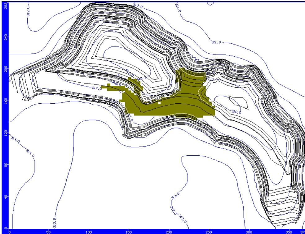
Figure 20: Drying Pattern for decreased recharge (140mm/year) with Evapotranspiration set to 300mm/year.
