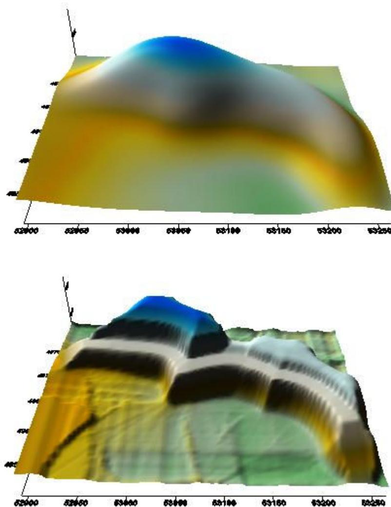
Figure 14: Defined water table compared to Hummock Topography (8x Vertical Exaggeration). Given that zone one required so little recharge to remain wetted and 1.5m was the desired depth to maintain the water table 1.5m was chosen as the depth to model with the hummock undefined.
