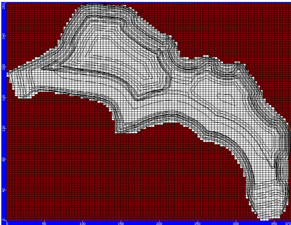
Figure 10: Constant heads assigned for cases 2-5, plan view of layer 1.
