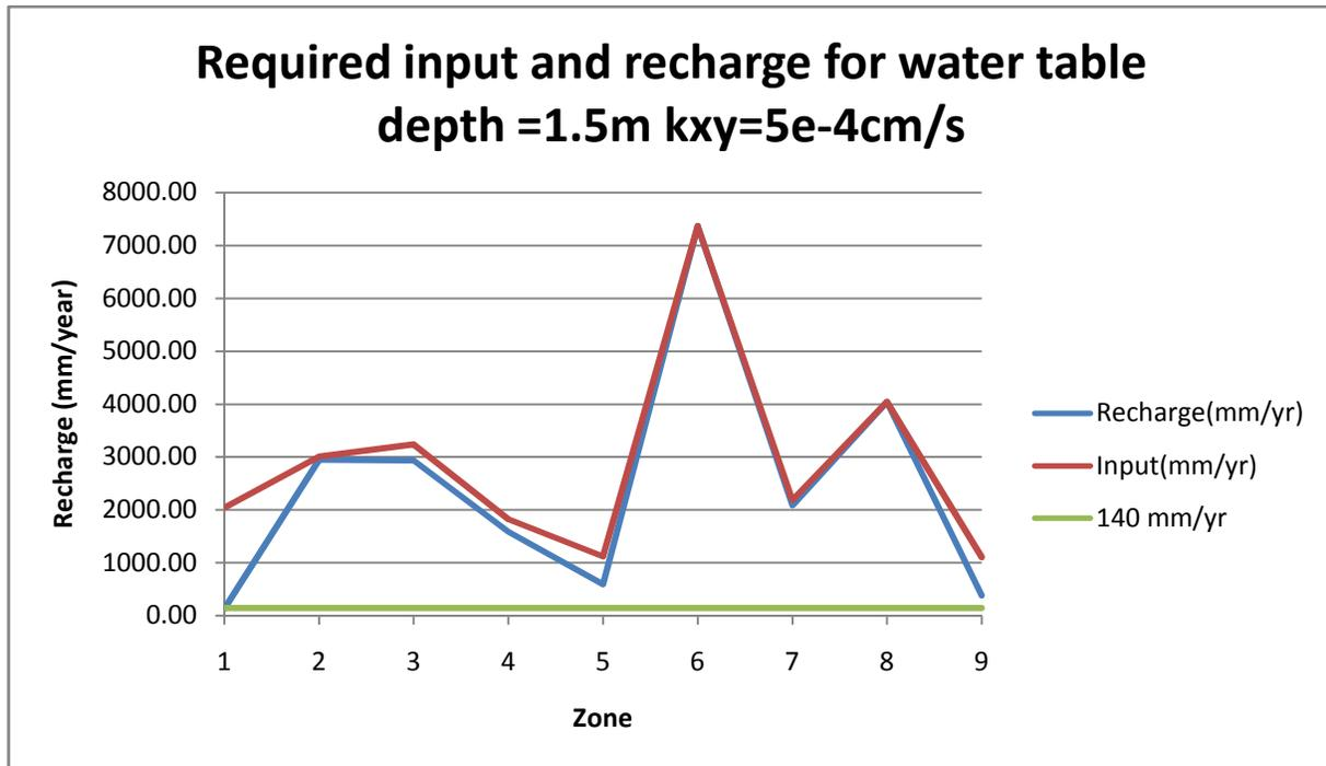
Figure 12: volumes for hummock with 1.5m depth constant water table  $k_{xy} 5 \times 10^{-4} \text{cm/s}$ .
