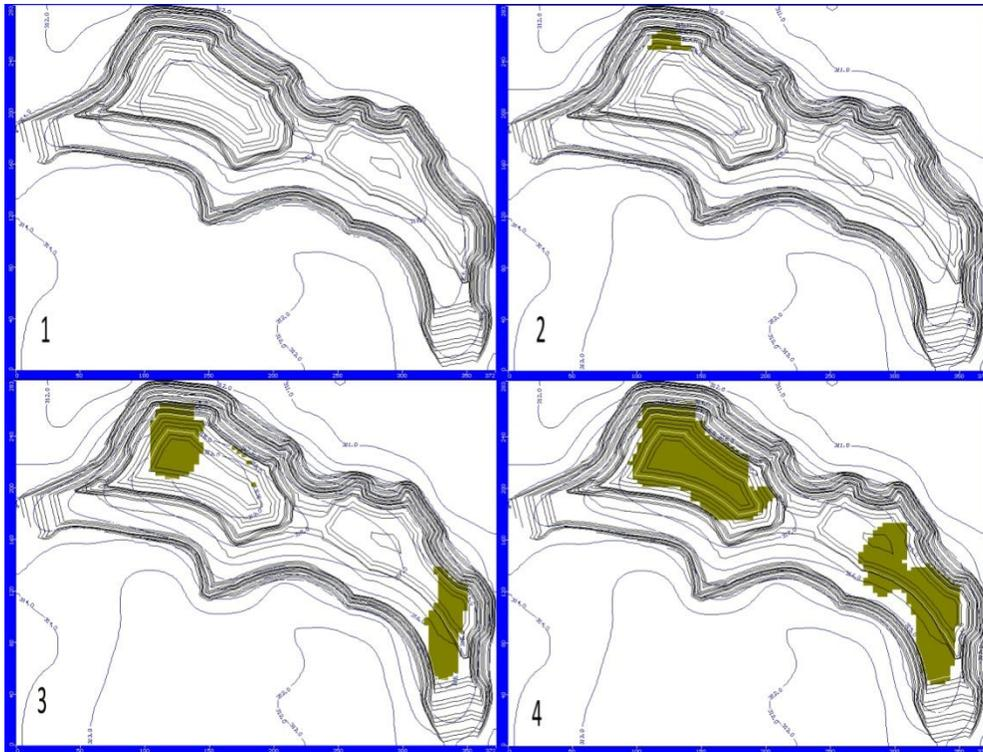
Figure 15: Dry cell overlay for case 2, 1.5m water table depth.  $K=1.0 \times 10^{-5} \text{cm/s}$ (1),  $1.25 \times 10^{-5} \text{cm/s}$ (2),  $1.5 \times 10^{-5} \text{cm/s}$ (3),  $2.0 \times 10^{-5} \text{cm/s}$ (4).
