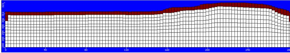
Figure 9: Constant heads assigned for case 1, section view through column 34.
