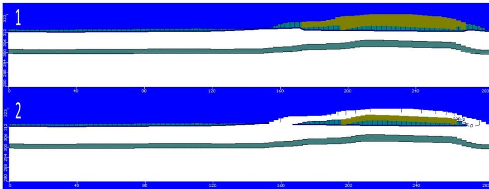
Figure 19: Section lines through column 34 for case 3, water table depth 1.5m  $K_{sand}=5.0 \times 10^{-4} \text{ cm/s}$ ,  $K_{cover}=1 \times 10^{-5} \text{ cm/s}$  (1),  $K_{sand}=5.0 \times 10^{-4} \text{ cm/s}$ ,  $K_{cover}=1 \times 10^{-6} \text{ cm/s}$  (2)
