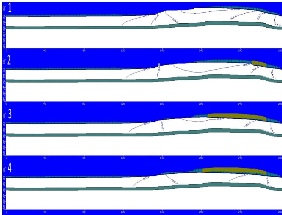
Figure 16: Section lines through column 34 for case 2, water table depth 1.5m  $K=1.0 \times 10^{-5} \text{ cm/s}$ (1),  $K=1.25 \times 10^{-5} \text{ cm/s}$ (2),  $1.5 \times 10^{-5} \text{ cm/s}$ (3),  $2.0 \times 10^{-5} \text{ cm/s}$ (4).
