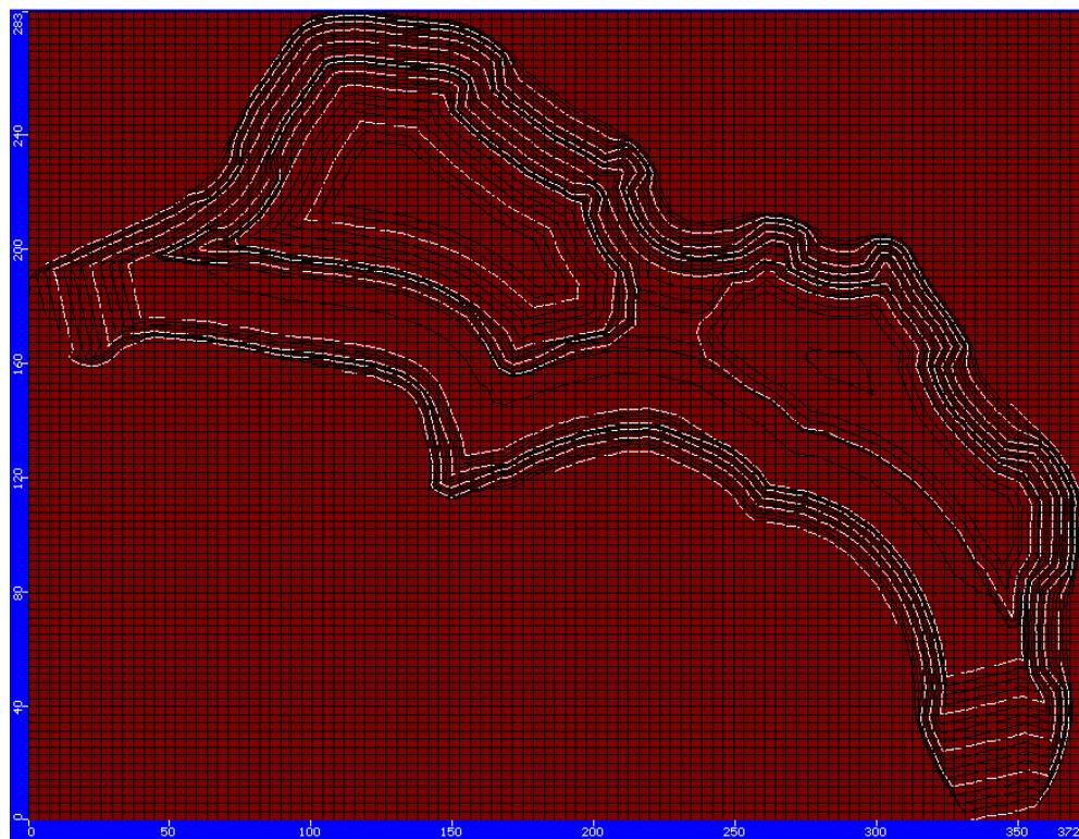
Figure 8: Constant heads assigned for case 1, plan view of layer 1.
