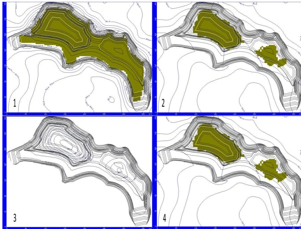
Figure 18: Dry cell overlay for case 3, 1.5m water table depth.  $K_{sand} = 5.0 \times 10^{-4} \text{ cm/s}$ ,  $K_{cover} = 1 \times 10^{-5} \text{ cm/s}$ , Layer 1(1),  $K_{sand} = 5.0 \times 10^{-4} \text{ cm/s}$ ,  $K_{cover} = 1 \times 10^{-5} \text{ cm/s}$ , Layer 2 (2),  $K_{sand} = 5.0 \times 10^{-4} \text{ cm/s}$ ,  $K_{cover} = 1 \times 10^{-6} \text{ cm/s}$ , Layer 1 (3),  $K_{sand} = 5.0 \times 10^{-4} \text{ cm/s}$ ,  $K_{cover} = 1 \times 10^{-6} \text{ cm/s}$ , Layer 2 (4).
