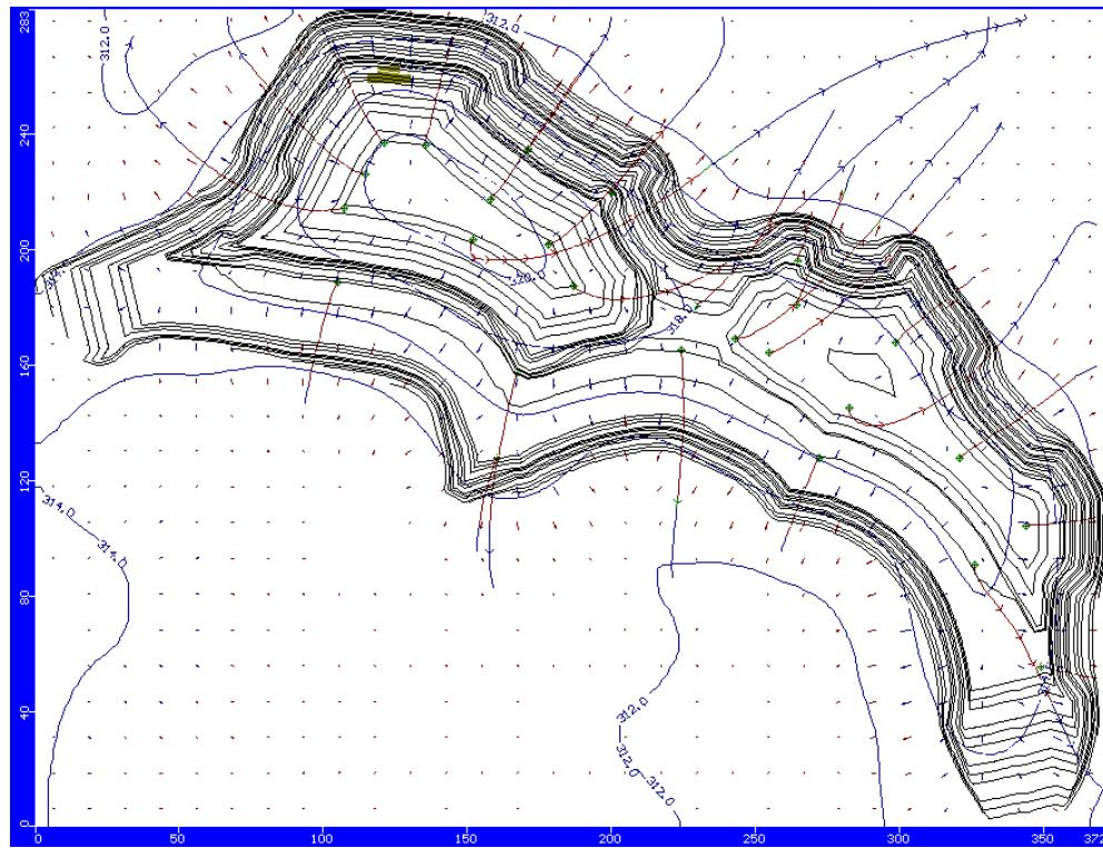
Figure 13: Flow velocity vectors and pathlines for defined water table 1.5m deep,  $K_{xy} = 5 \times 10^{-4}$  cm/s.
