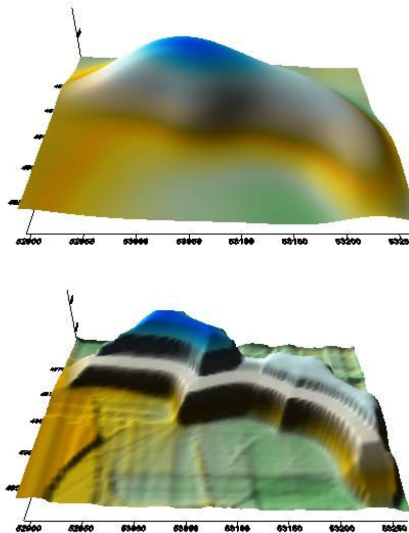
Figure 14: Defined water table compared to Hummock Topography (8x Vertical Exaggeration).
