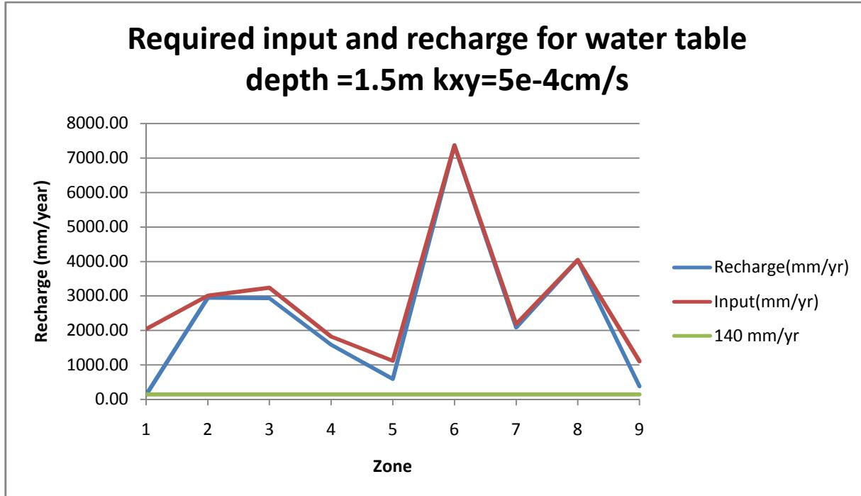
Figure 12: volumes for hummock with 1.5m depth constant water table  $k_{xy} 5 \times 10^{-4}$  cm/s.
