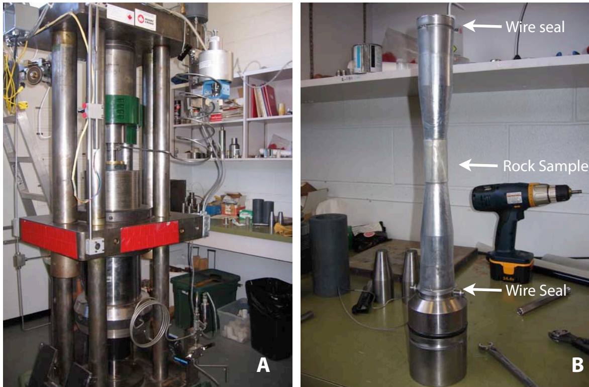
Figure 2. A. LSR detail with sample assembly inserted and pore fluid system installed. B. Sample assembly detail with fractured 30 mm diameter sample, polyolefin jacket and wire seals in place.
