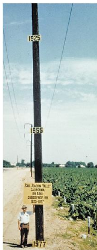
Figure 17: Mendota, California subsidence due to groundwater withdrawal from 1925 – 1977 (Galloway et al. 1999).
