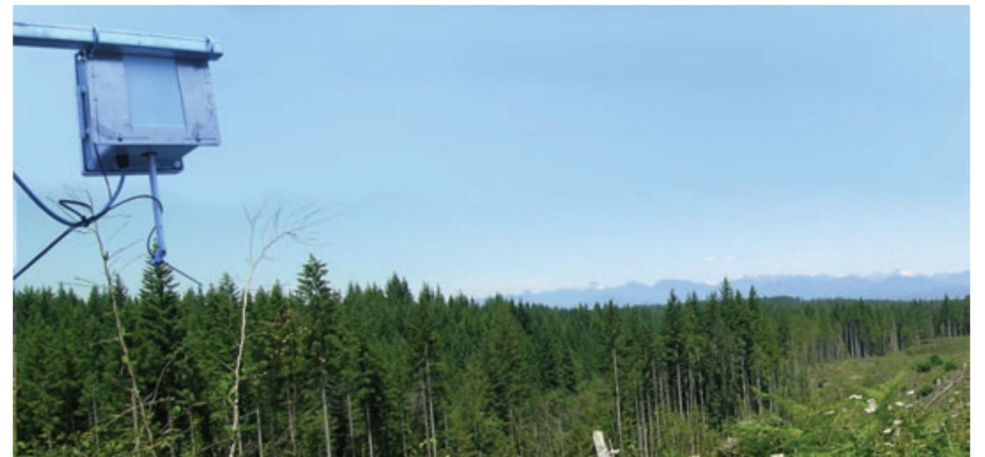
View from the top of the FLUXNET-Canada Campbell River tower with the automated spectro-radiometer measuring canopy reflectance every 15 minutes, 24 hours a day.
