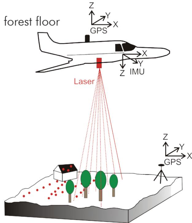
Schematic diagram showing how an airborne LiDAR system works. A laser pulse is sent from the aircraft to the ground and the beams are returned from either the ground surface or the forest canopy. Each LiDAR pulse is approximately 15 cm in diameter and is horizontally spaced at less than 1 m apart over the entire landscape.
