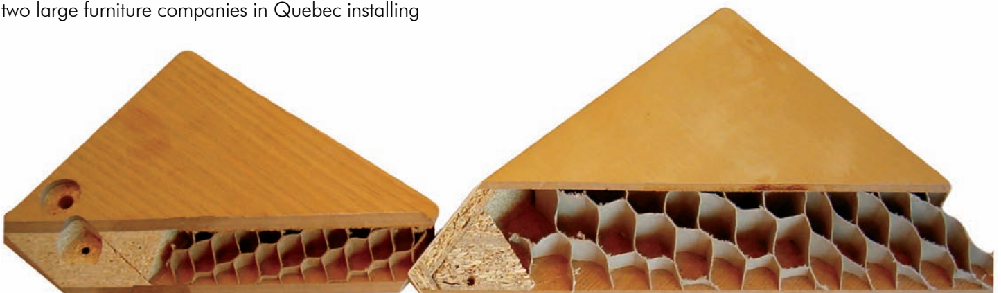
Honeycomb sandwich panels can be found in many imported thick furniture items. Left: a local custom-built veneered tabletop, and right: a mass-produced plastic coated tabletop.
