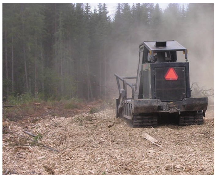
Figure 2: Gyro Trac GT-25 mulching windrow of waste material
